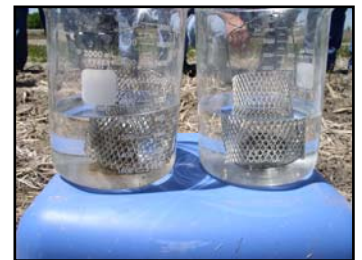
Tilled (breaking apart dirtier) No-till (In tact, cleaner)
